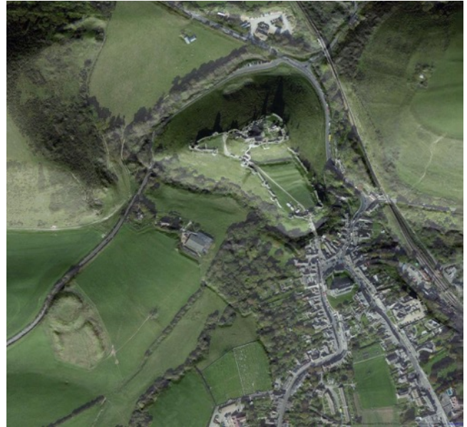
Air photo of Corfe Castle and, to the south west, The Rings . The Bing airphoto overlaid with a semitransparent LiDAR image done with the hillshading set to match the lighting in the air photo. Not bad in giving a bit more 'depth' to the air photo but doesn't quite highlight the earthworks as much as the same image done with the hillshading at a different angle.
